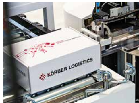
A careful grip: Toru grasps cartons by means of a suction unit.
