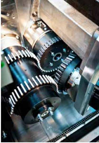
Rollers in the Multi Segment Maker: Its modular concept enables the MSM to be adapted to specific customer requirements.
