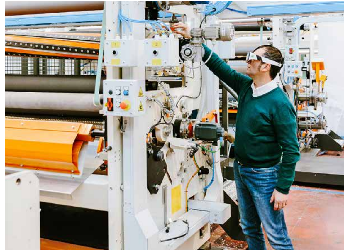
Insight: The wearer of the camera can select menu points on the display in front of his eyes by looking at them directly.
